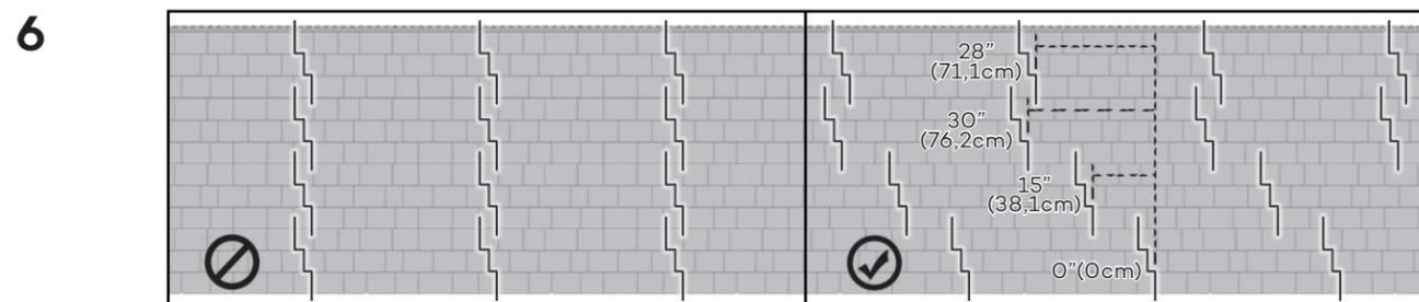
Alternate the joints between rows. For a nicer look, we suggest alternating the cutting distance of the first section of every row from 0" (0cm) - 15" (38,1cm) - 30" (76,2cm) - 28" (71,1cm).
