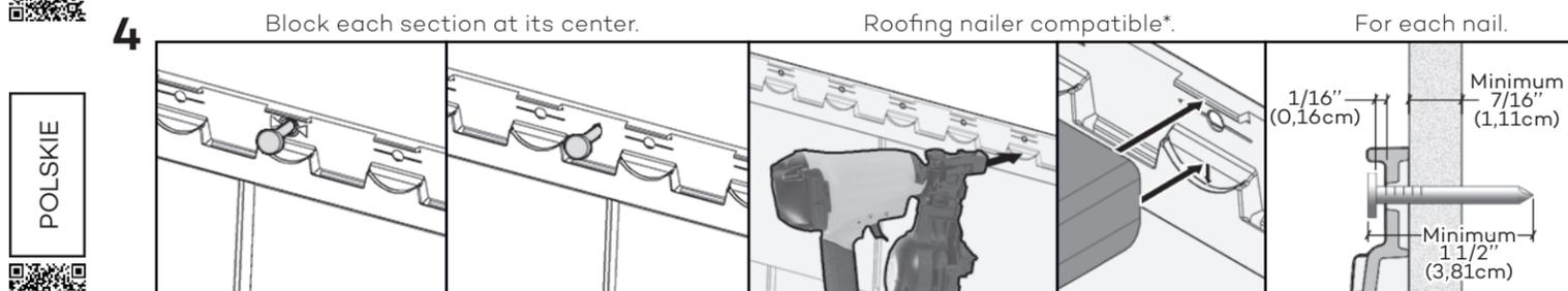
When installing a full section, nail in the center hole first. When installing a cut section, nail in its center. For each nail, leave a gap between nail head and section. When using a roofing nailer, adjust its tip at the highest position and the air pressure according to the substrate in order to leave the required gap.
