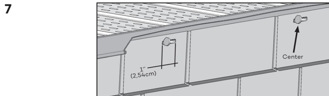
If you need to attach the section in an area other than the installation hole, create a 1" (2,54 cm) long slot to allow nailing. Always nail in the middle of the slot.
